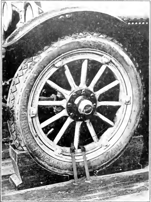
FIG. 6 METAL STRAPS AND ANOTHER KIND OF WOODEN BLOCK USED IN THE "TIE-DOWNS"
